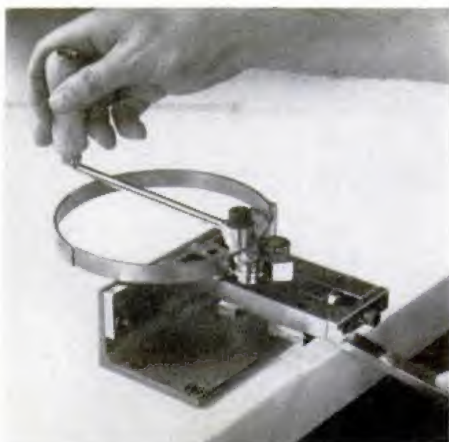
TO ROLL RINGS , anvils are replaced with a crank-operated roller. Lever pressure determines the radius
